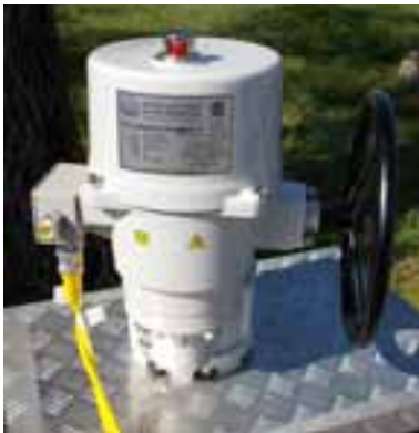
Custom Remote Mounted MCC P12-383 3 Phase Industrial Actuator with custom wiring harnesses
