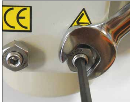
CW Mechanical Stop CLOSE, 0°, 4mA, Red Cams
