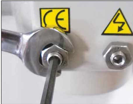
CCW Mechanical Stop OPEN, 90°, 20mA, Green Cams
