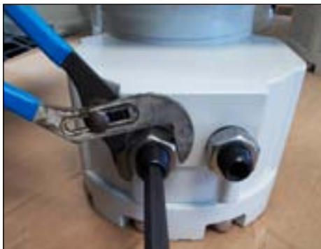
CCW Mechanical Stop
