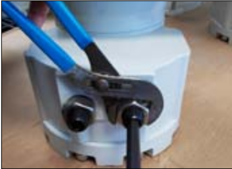
CW Mechanical Stop
