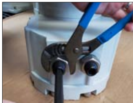
CCW Mechanical Stop
