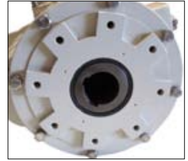
The actuator is shown in its fully CW position. This view of actuator showing the two drive keyways machined into the female drive socket.
