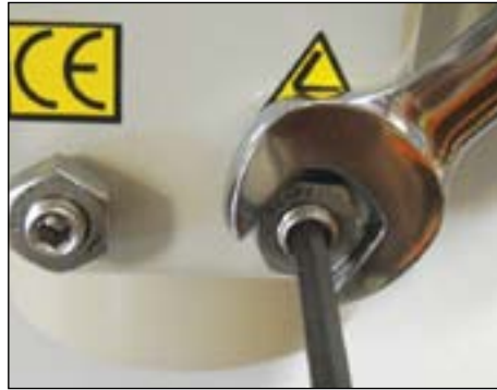
CW Mechanical Stop CLOSE, 0°, 4mA, Red Cams
