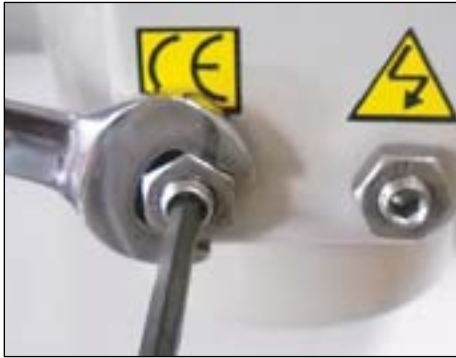
CCW Mechanical Stop OPEN, 90°, 20mA, Green Cams
