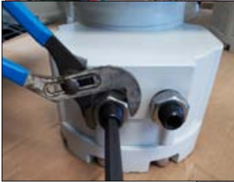
CCW Mechanical Stop
