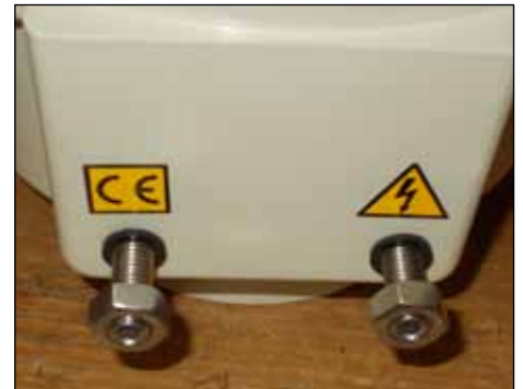
Mechanical Stop Adjustment Positions
