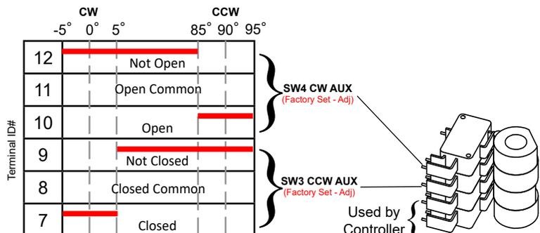
On/Off Switch/Cam arrangement shown
