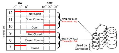
On/Off Switch/Cam arrangement shown
