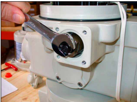
Loosen lock nut. Refer to step 4
