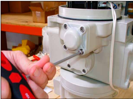
Remove adjustment housing cover. Refer to step 3
