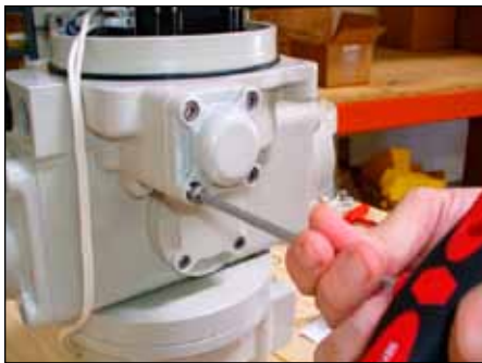
Remove adjustment housing cover. Refer to step 3
