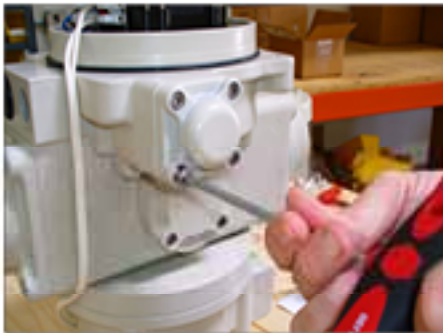
Remove adjustment housing cover. Refer to step 3
