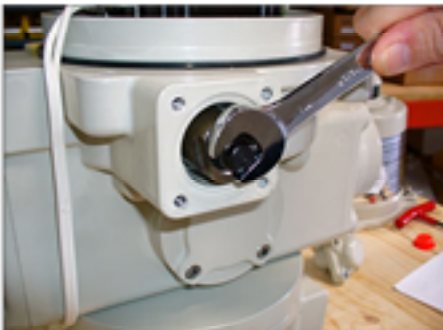
Loosen lock nut. Refer to step 4
