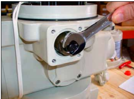
Loosen lock nut. Refer to step 4
