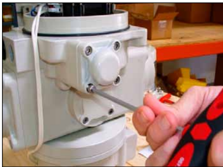
Remove adjustment housing cover. Refer to step 3
