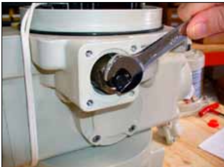
Loosen lock nut. Refer to step 4
