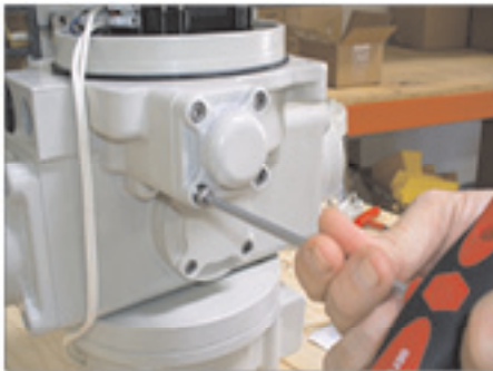
Remove adjustment housing cover. Refer to step 3
