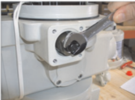
Loosen lock nut. Refer to step 4
