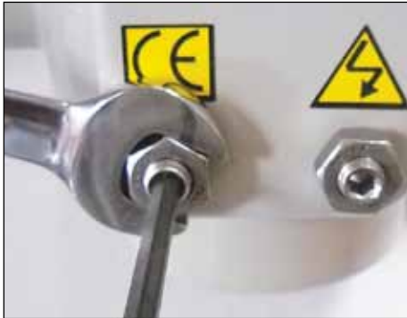
CCW Mechanical Stop OPEN, 90°, 20mA, Green Cams
