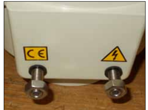
Mechanical Stop Adjustment Positions
