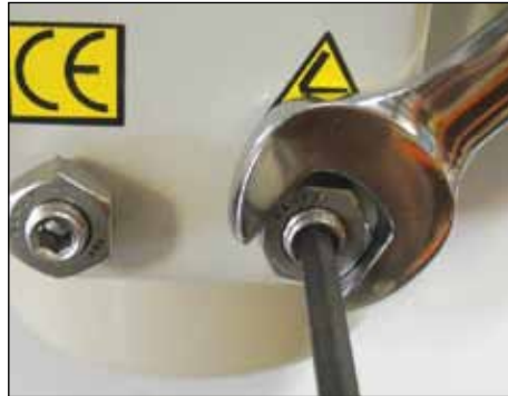
CW Mechanical Stop CLOSE, 0°, 4mA, Red Cams
