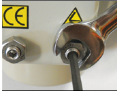
CW Mechanical Stop CLOSE, 0°, 4mA, Red Cams
