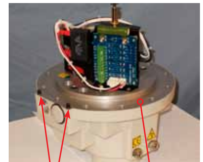
Alignment pins/holes (refer to note 6) Mating Surfaces (refer to note 5, 6)
