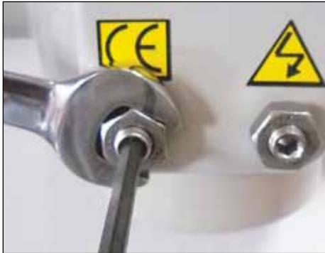
CCW Mechanical Stop OPEN, 90°, 20mA, Green Cams
