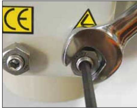
CW Mechanical Stop CLOSE, 0°, 4mA, Red Cams
