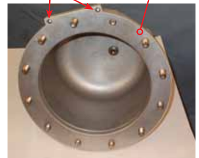
Alignment pins/holes (refer to note 6) Mating Surfaces (refer to note 5, 6)
