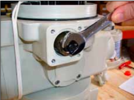
Loosen lock nut. Refer to step 4
