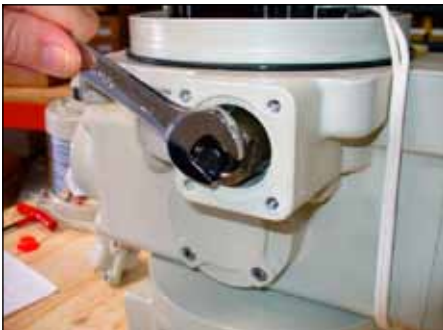
Loosen lock nut. Refer to step 4
