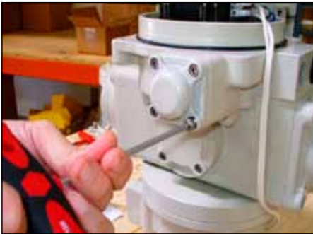
Remove adjustment housing cover. Refer to step 3
