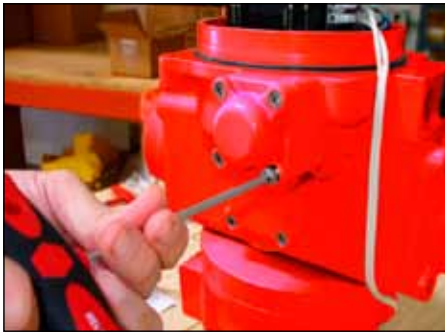
Remove adjustment housing cover. Refer to step 3
