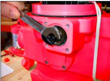
Loosen lock nut. Refer to step 4
