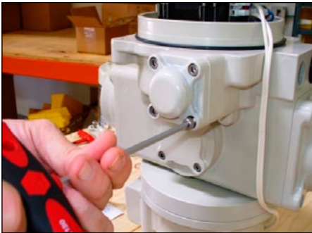
Remove adjustment housing cover. Refer to step 3
