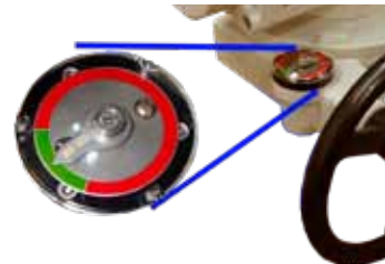
Location indicator shown in the UNLOADED operational position.
