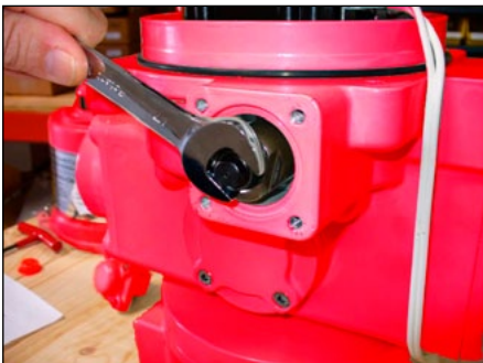
Loosen lock nut. Refer to step 4
