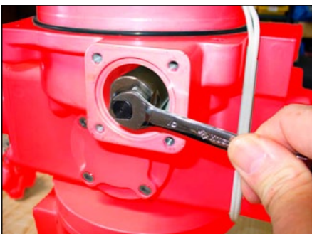
Turn the adjustment nut to adjust UNLOADED position. Refer to step 4
