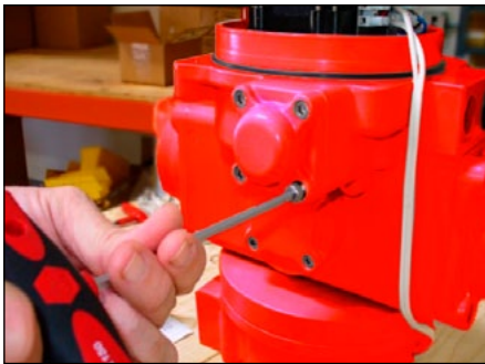
Remove adjustment housing cover. Refer to step 3
