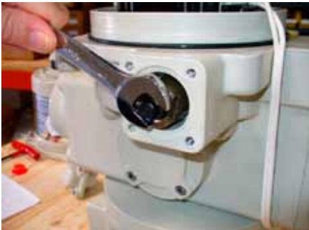
Loosen lock nut. Refer to step 5
