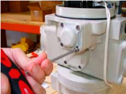
Remove adjustment housing cover. Refer to step 4
