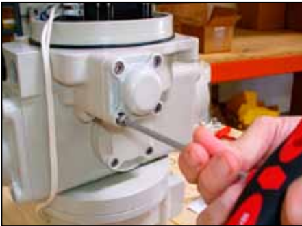
Remove adjustment housing cover. Refer to step 3
