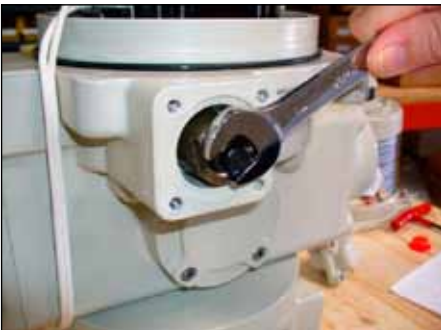
Loosen lock nut. Refer to step 4
