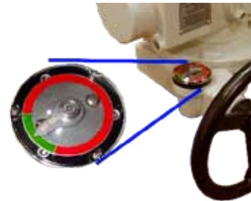
Location indicator shown in the UNLOADED operational position.
