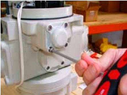
Remove adjustment housing cover. Refer to step 4
