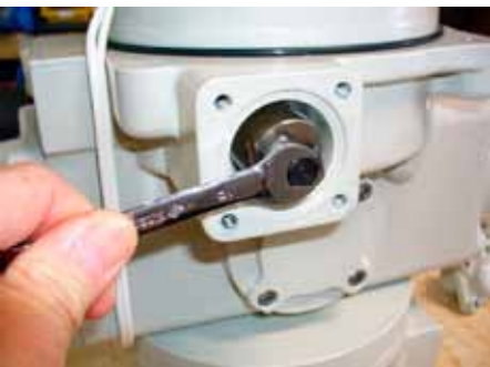
Turn the adjustment nut to adjust UNLOADED position. Refer to step 5
