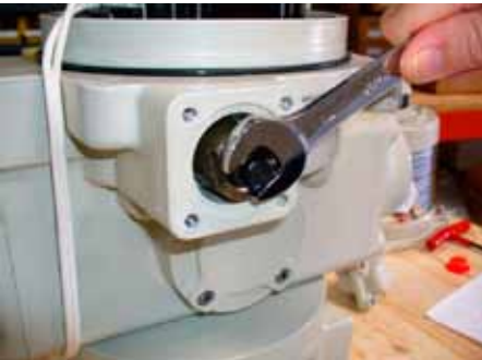
Loosen lock nut. Refer to step 5
