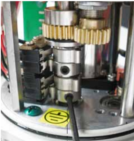
Cam 1 Indicator/ Camshaft movement Output Drive movement
