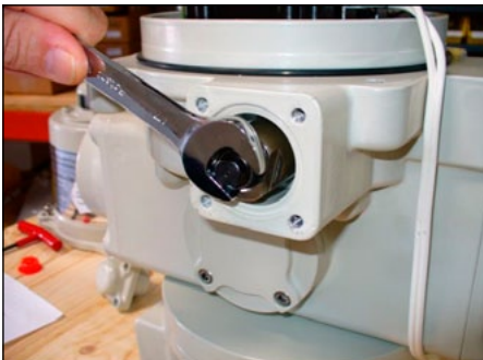
Loosen lock nut. Refer to step 4
