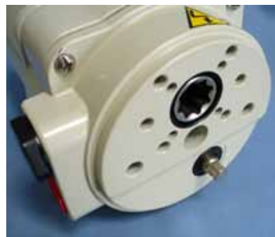
ISO F03/05 Mounting Detail, 8 point 14mm female drive, and 8mm socket override on P1, P1.B, and P1.C Series actuators.
