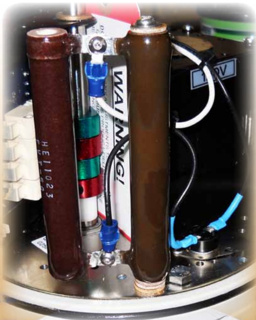
85W Heater bank installed in P2 series actuator
