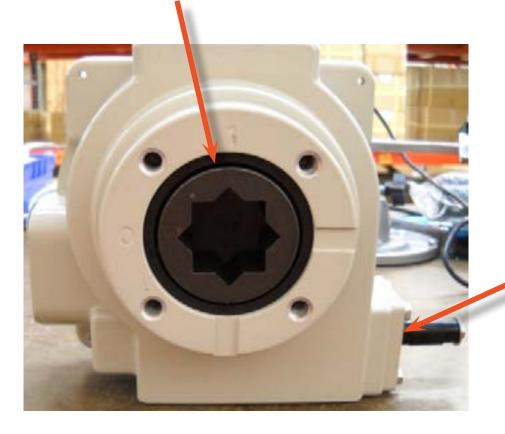
The override shaft receives the same attention to surface finish at the O-Ring seal contact area.
