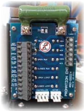
Additional Auxiliary Switches on Ruggedboard switch card
