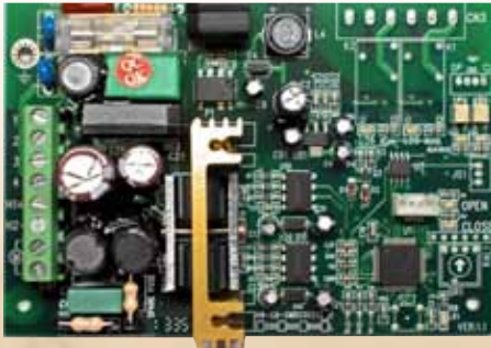
Extended Duty Control Board supplies power and control to the 90vdc motor.
